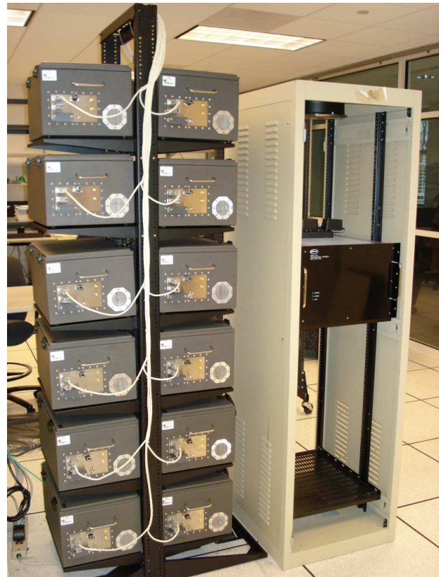
Figure 1: Assembly and connection of the shielded enclosures and RF switch.
