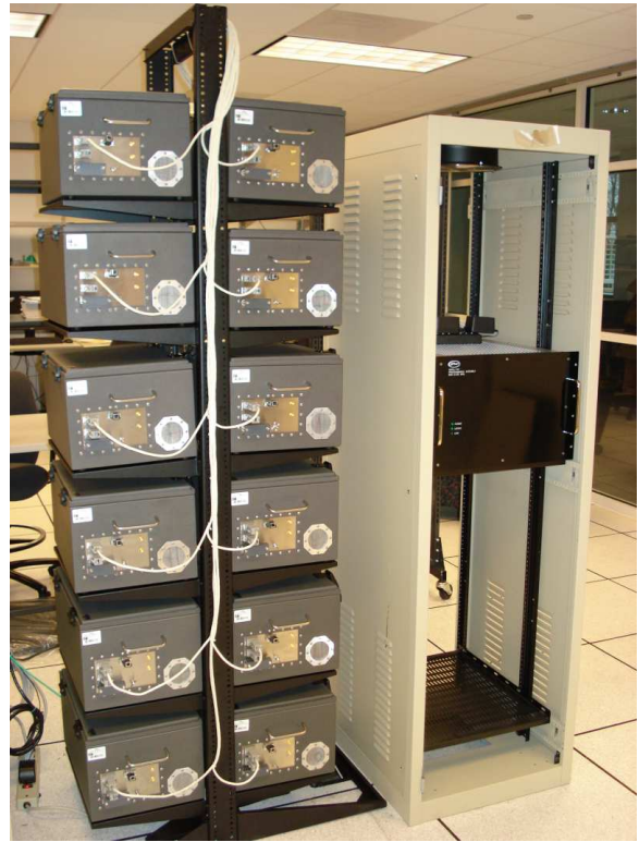
Figure 1: Assembly and connection of the shielded enclosures and RF switch.
