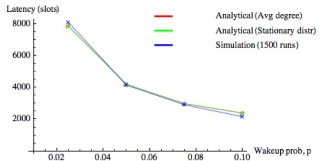
**Figure 5:** Comparison between approximation formulas and simulations of average end-to-end latency suffered by duty cycling random walks between the farthest pair of nodes on the 100 node graph shown in Fig. 4 against different values of  $p$ .
