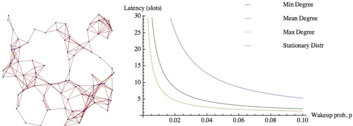
**Figure 4: A random geometric graph with  $n = 100$ ,  $r = 0.15$ , and  $p = 0.1$ ; and the average per-hop latency according to various bounds and approximation formulas: Min and Max curves are given by Equation 3; the Mean curve is given by per-hop component of  $\tilde{\mathbf{L}}_{s,t}^{(1)}$  and Stationary Distribution curve refers to the per-hop component of  $\tilde{\mathbf{L}}_{s,t}^{(2)}$**
