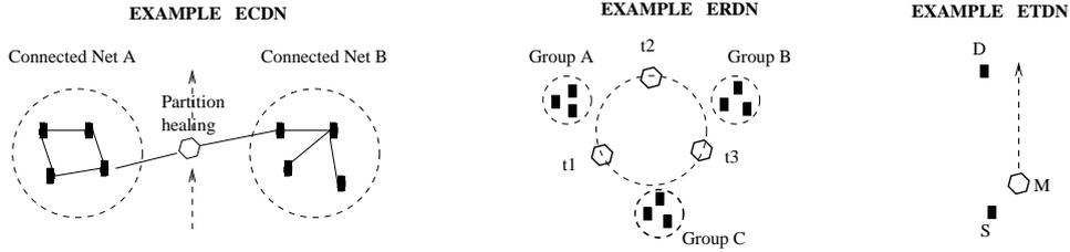
**Figure 1:** Partition healing (left) is an example of Eventually Connected Dynamic Network (ECDN), and a UAV sequentially connecting pairs of battalions (center) is an example of Eventually Routable Dynamic Network (ERDN). A message ferry (right) is a simple example of an Eventually Transportable Dynamic Network (ETDN).
