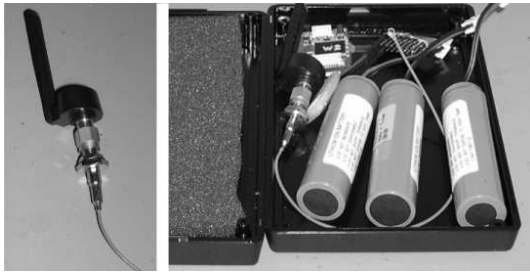
Figure 2: Long range iMote with rechargeable batteries.
